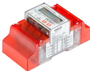
Meter 3f PRO380-Mb x/5A M-Bus Three-phase electricity meter indirect measurement, MID approved. Pulses & M-Bus data output - 3x230V/400V, 100A.
