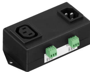
PowerEgg2 110/230 V single phase, max. load 8 A
