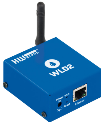
WLD2 WLD2 is a WiFi/Ethernet water leak detector with support for WWW, SNMP and PoE. To detect leaking liquids, it uses 4 sensing cables.
